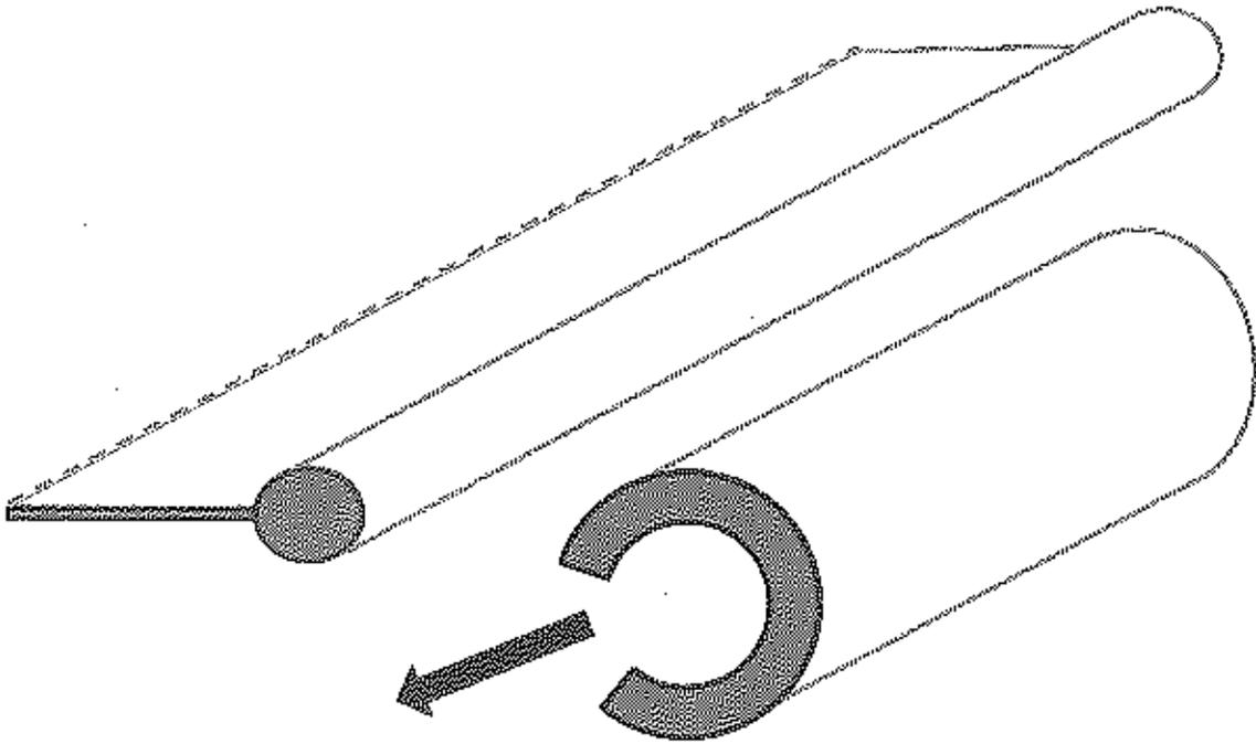
The zipper pulls out of the channel on the top portion of the arch only. The sides of the arch are tight.
