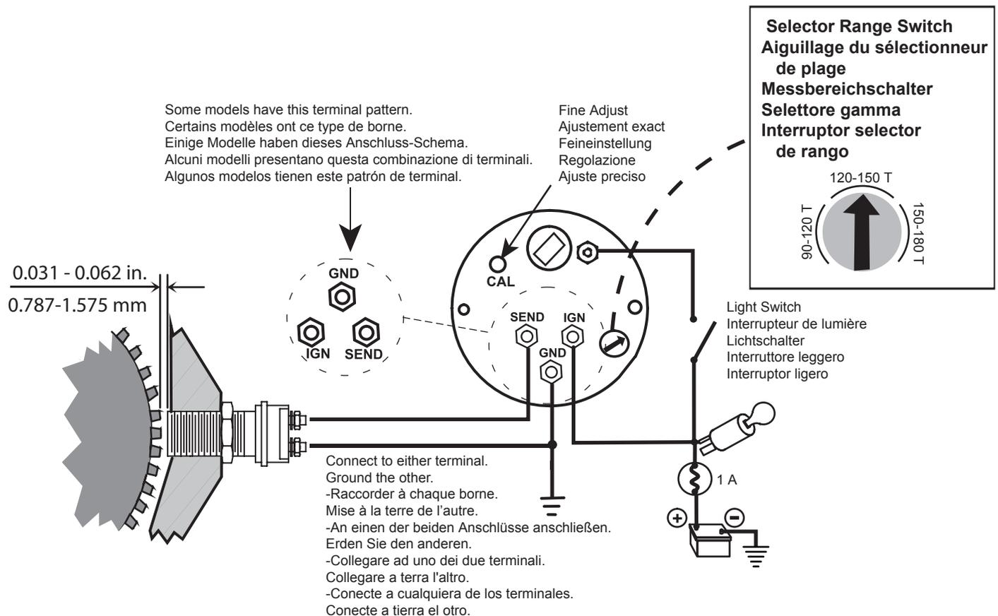
Set Selector Range Switch with the arrow pointing at the gear range that includes the number of teeth on your flywheel.
