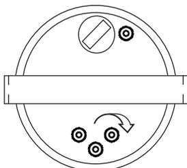
Electrical connections tighten 0.70 nm max. (100 in. oz.)
