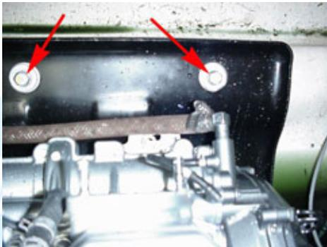
4.6 (Below) Flip the engine and bedplate onto its side and remove the four bolts securing the engine to the bed plate. Flip the engine and bed plate back and remove the engine from the hull.
