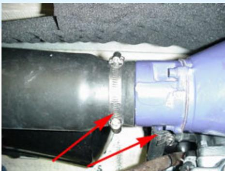
2.3 (Below) Remove the four allen head bolts securing the stinger pipe to the header pipe. Remove the stinger from the hull.
