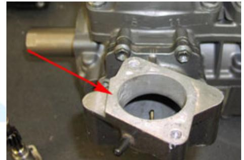
5.1 (Above) Remove the six nuts and twelve bolts securing the intake manifold to the engine. Remove the oil lines from the manifold.
