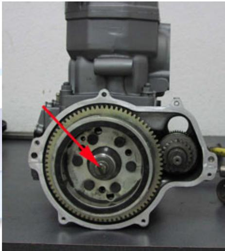
5.1 (Above) Remove the flywheel bolt. Remove the flywheel using a universal flywheel puller.
