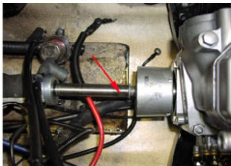
4.5 (Below) Remove the four 14mm engine mount bolts. Remove the engine from the hull.
