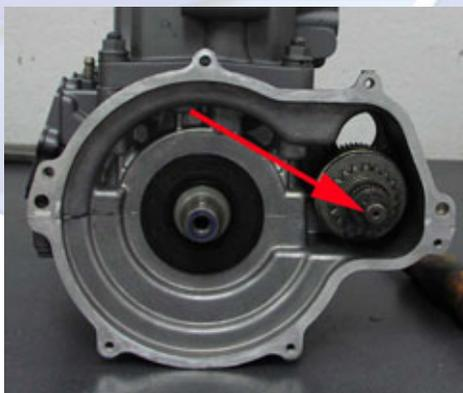
5.3 (Below) Remove the two 12mm bolts securing the starter to the engine.
