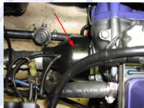
4.3 (Below) Remove the six 10mm bolts from the flywheel cover and remove the cover and leave it in the hull.
