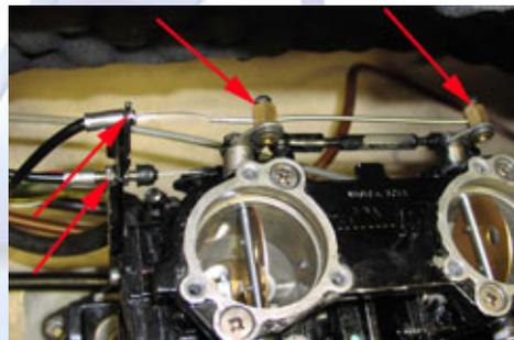
2.5 (Below) Remove the four 5mm bolts securing the carbs to the intake manifold. Remove the carbs from the hull.
