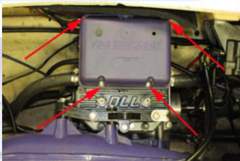
2.2 (Below) Remove the six 10mm bolts connecting the air box to the carbs. Remove the three 14mm bolts holding the air box and exhaust to the head.
