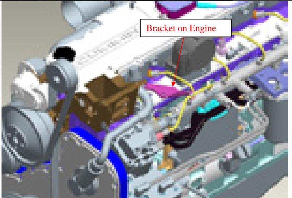
Tighten the bracket screws to the intake manifold cover plate.
