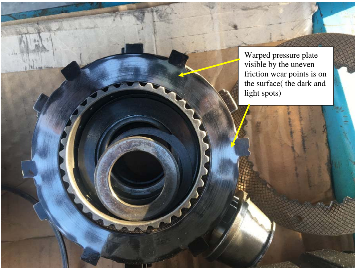
Figure #4- Warped clutch pressure plate.
