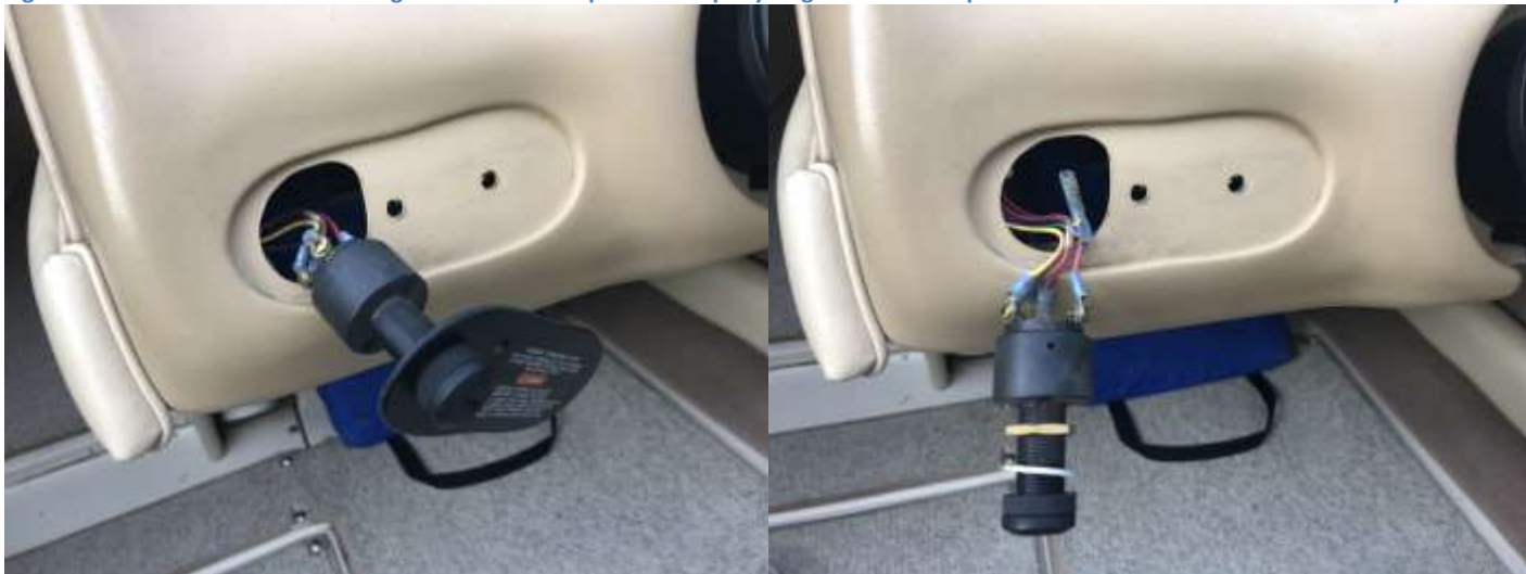
Figure 7: The kit comes with a new ignition switch. I opted to keep my original. Remove panel and leave wired to cable assembly.
