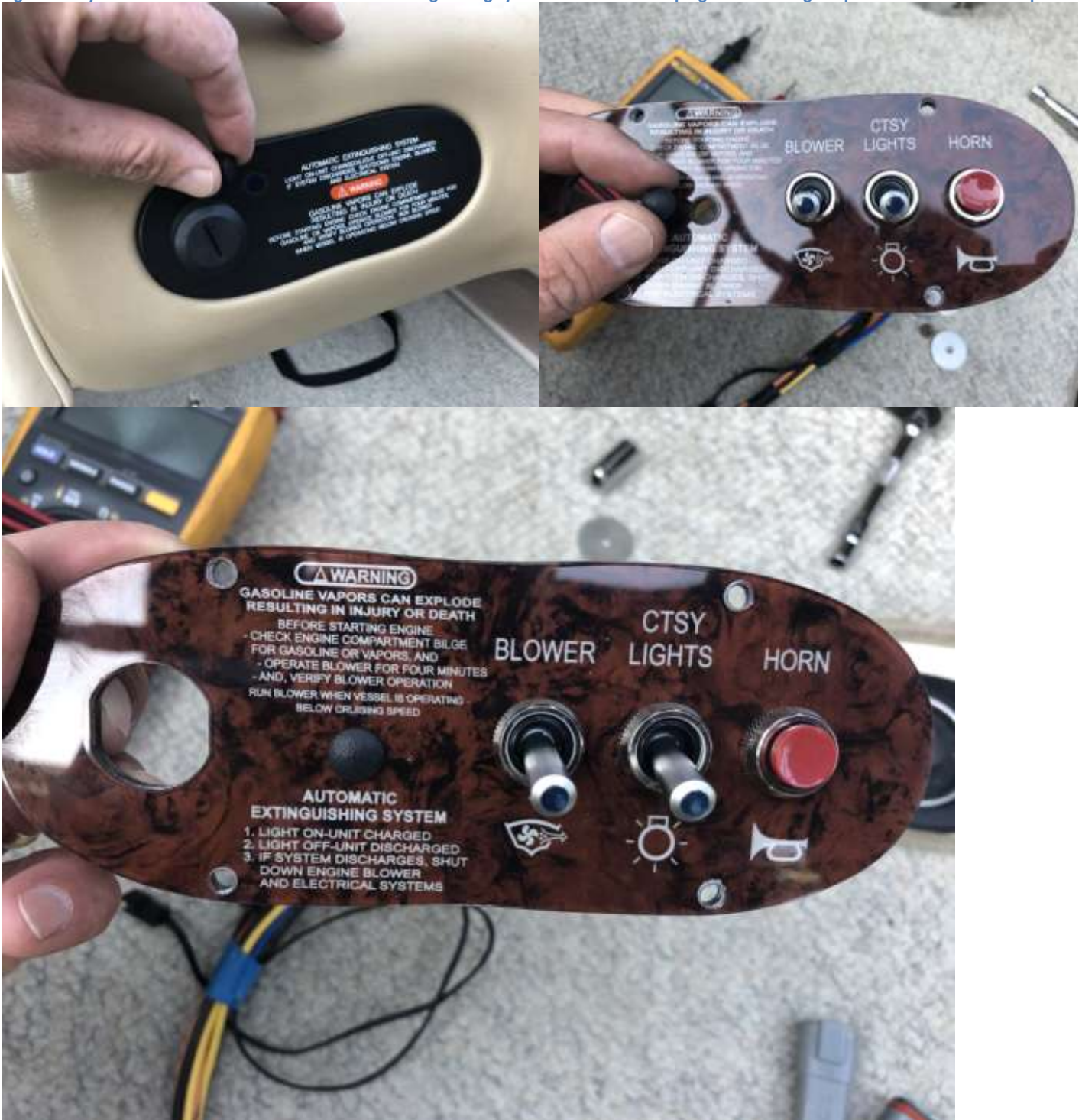
Figure 6: My install did not have the automatic fire extinguishing system. Remove small plug from the original panel and install in new panel.
