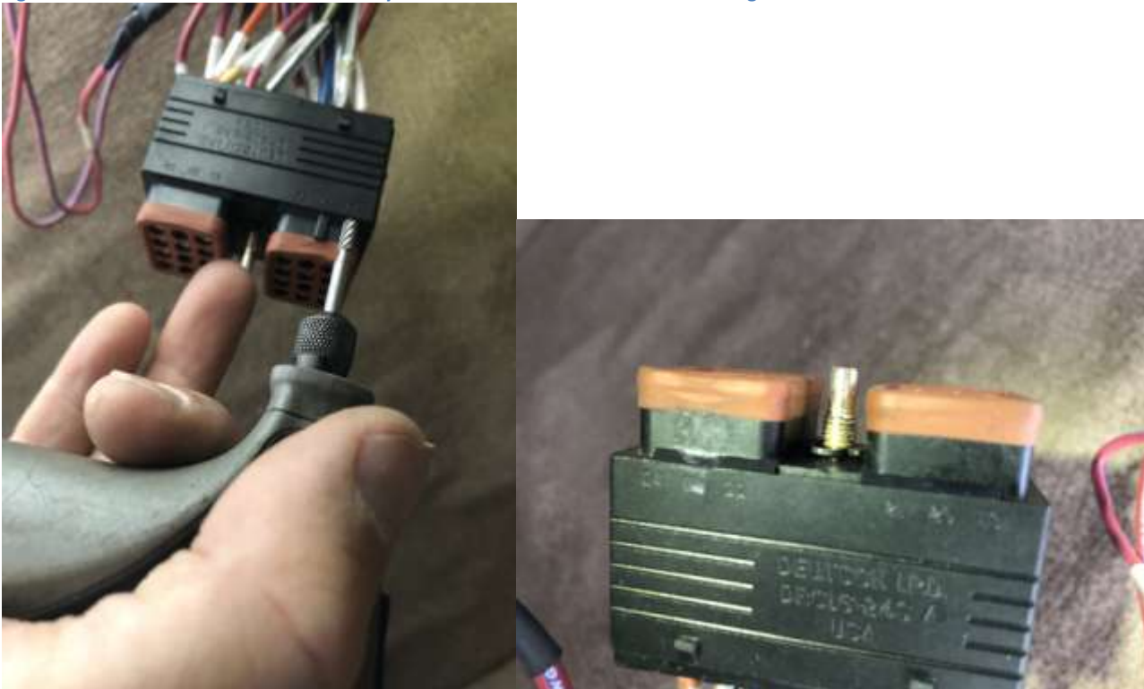
Figure 11: Used Dremel to remove mate key. Note: there is one on each terminal lug.
