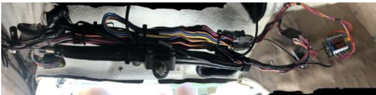
Figure 21: Panoramic of cable routing under helm.
