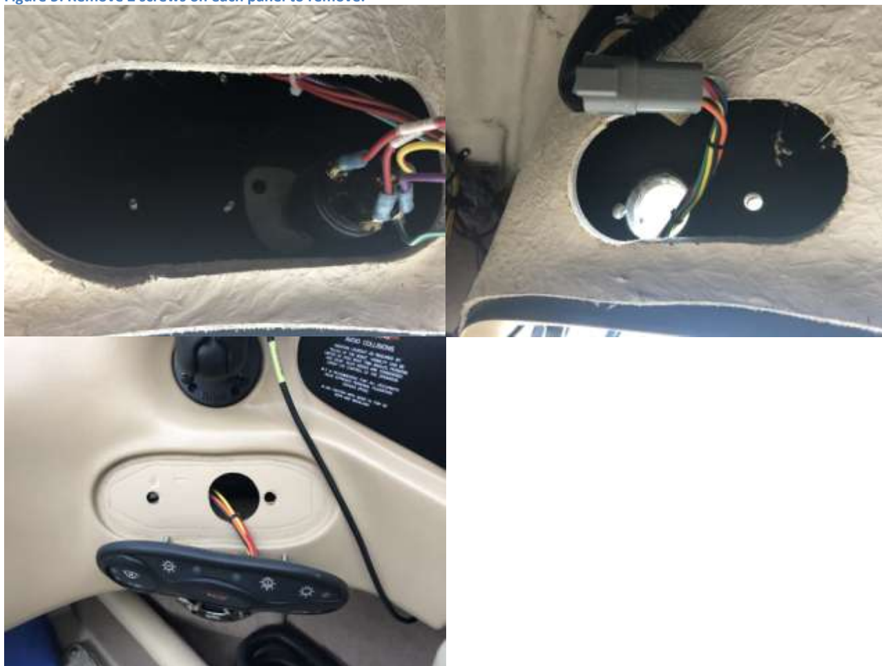
Figure 5: Remove 2 screws on each panel to remove.
