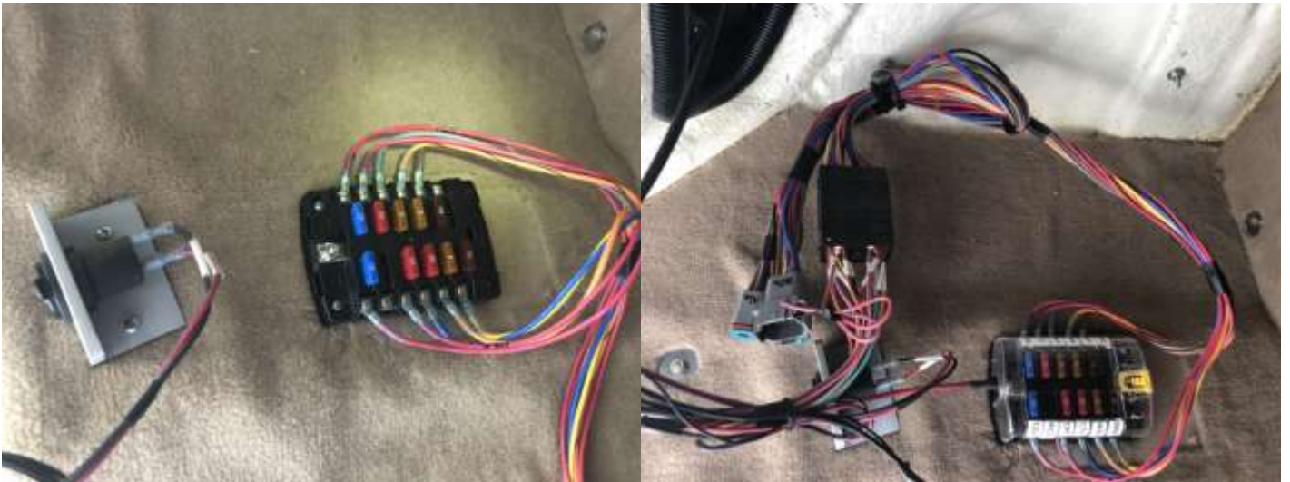
Figure 13: Installed new fuse block in same location as the original EIM, reusing the screws from the EIM removal. Installed cable hanger on available bolt and routed cable assembly over top of fuse block.
