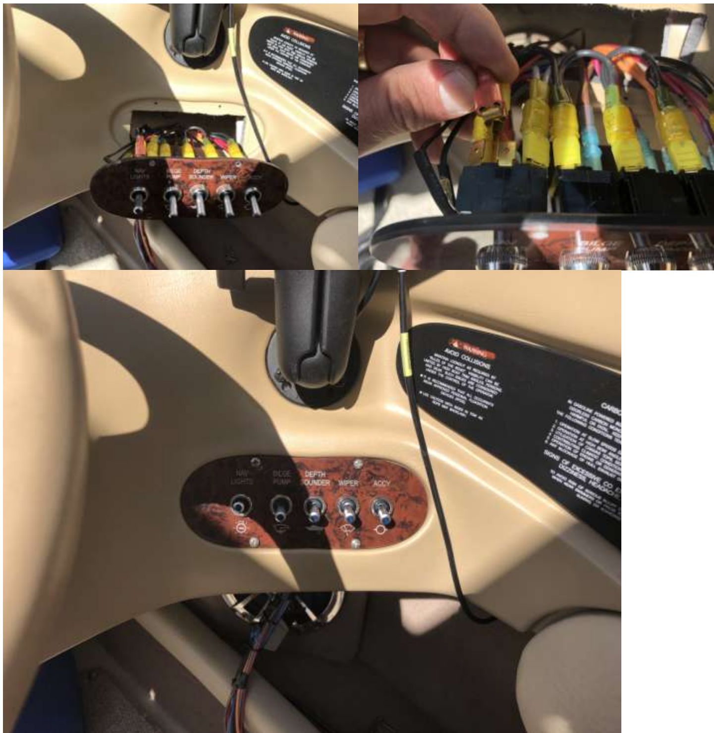
Figure 17: When installing the main switch panel, it was necessary to disconnect one terminal to fit through the cutout due to a slight interference. Remember to reconnect once the panel is installed.
