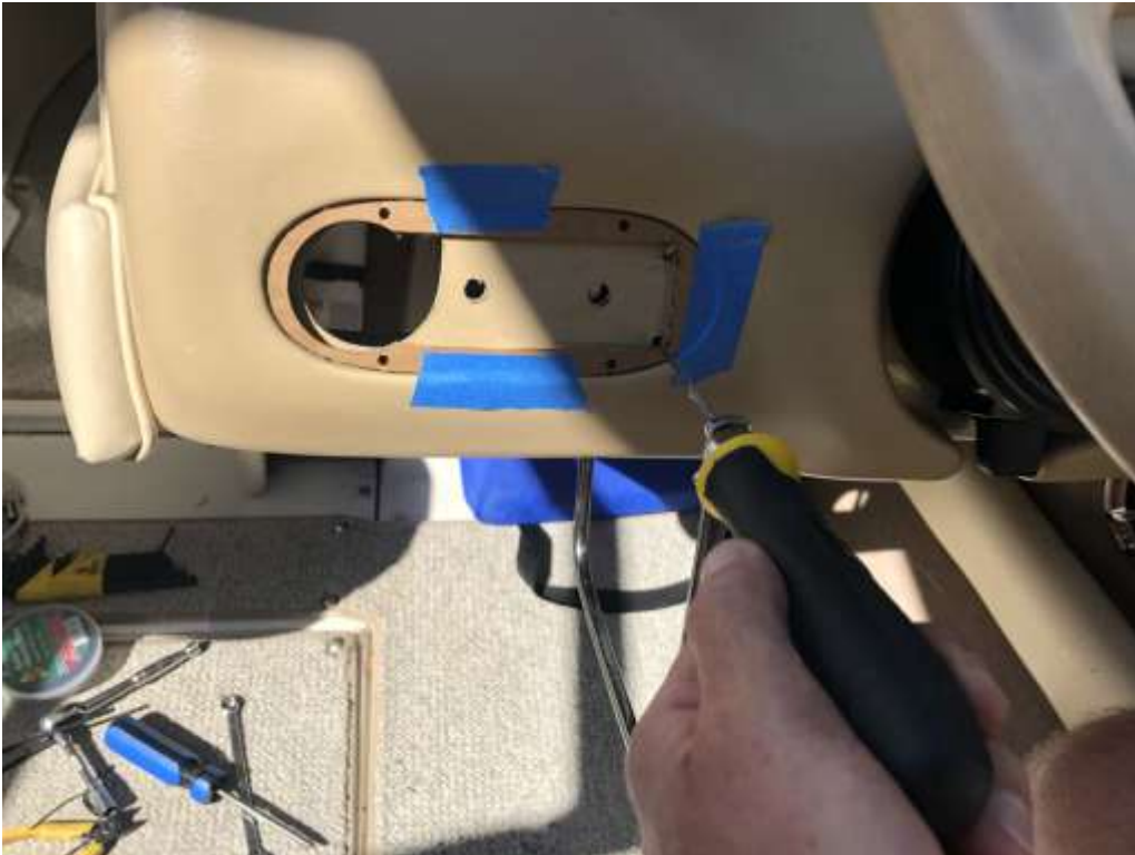
Figure 16: Used coping saw to cut slots. Worked perfectly! I am sure there are other methods, this one worked for me. The main peanut panel required cutting some of the fiberglass behind the dash panel. This just required drilling through the dash and rear fiberglass when drilling the holes. The coping saw cut both at the same time.
