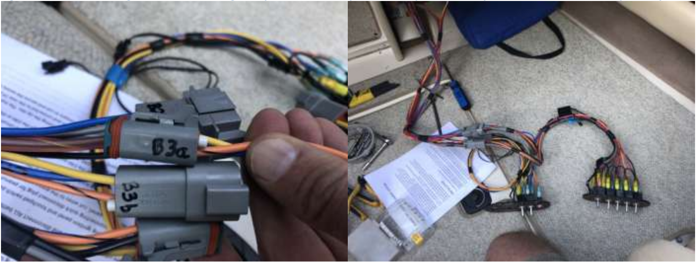
Figure 12: Before installing new EIM and cutting dash panel. I hooked up the entire system to verify correct function. Worked perfectly.
