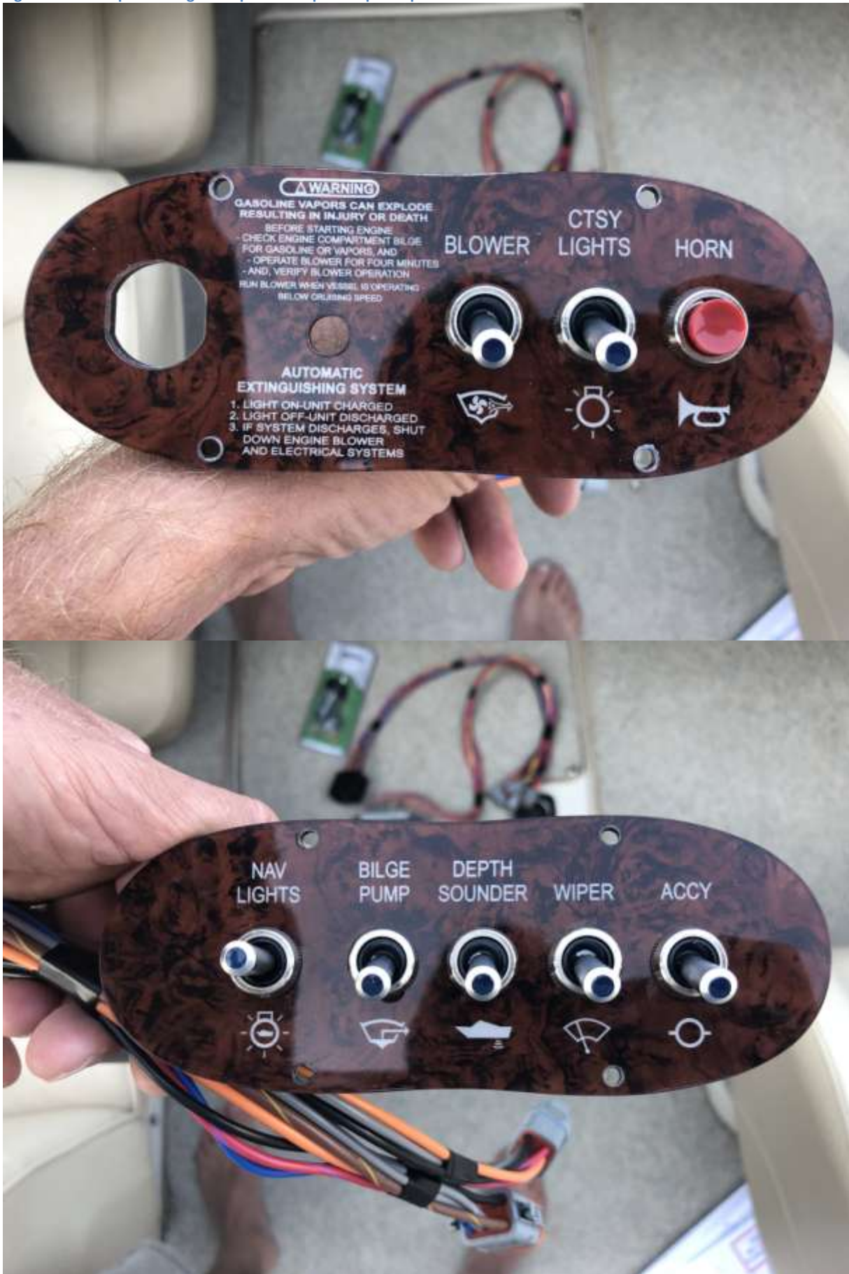
Figure 4: Close-up of new ignition panel and peanut pad replacement.
