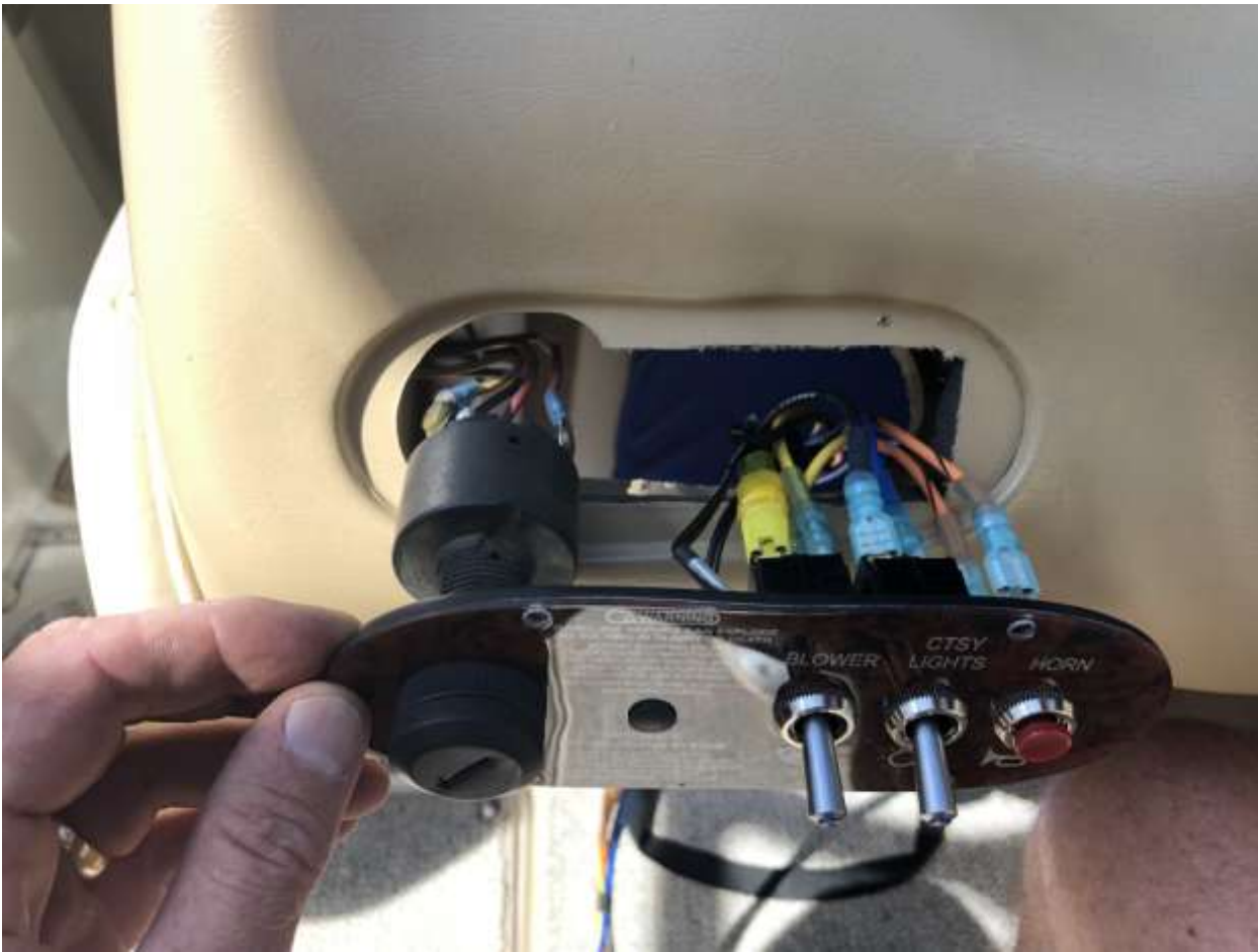
Figure 18: Install the ignition switch on new panel before installing.
