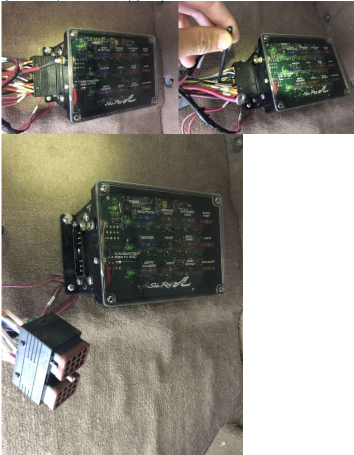
Figure 8: Remove EIM power wire then disconnect plug assembly with Allen wrench.
