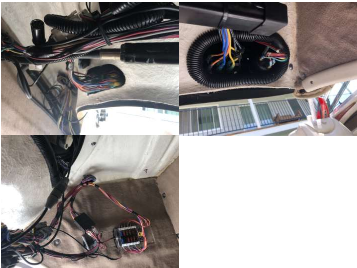
Figure 20: Routed all cables with existing wire bundles and secured with zip ties.
