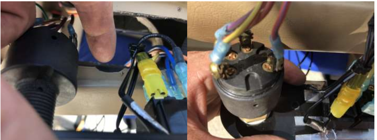
Figure 19: A small relief was needed to get the ignition panel to sit flat and flush. The wire interfering is seen in the second picture.
