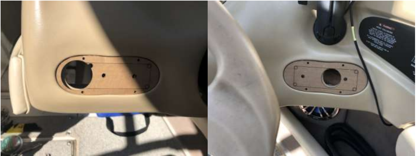
Figure 14: Installed drill/cut templates into dash panel.
