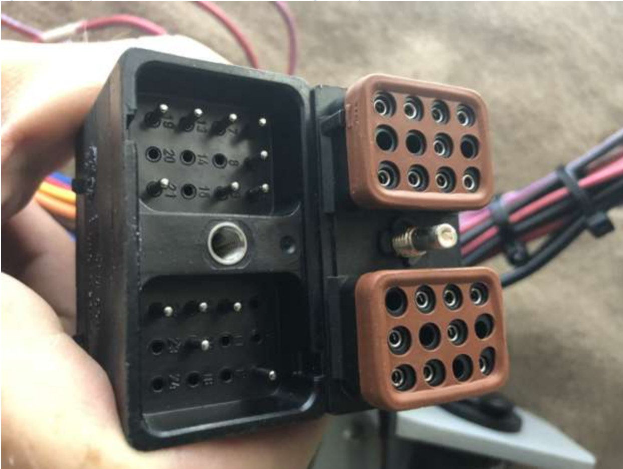
Figure 10: Plug key did not match as stated in instructions. Plug side requires modification.
