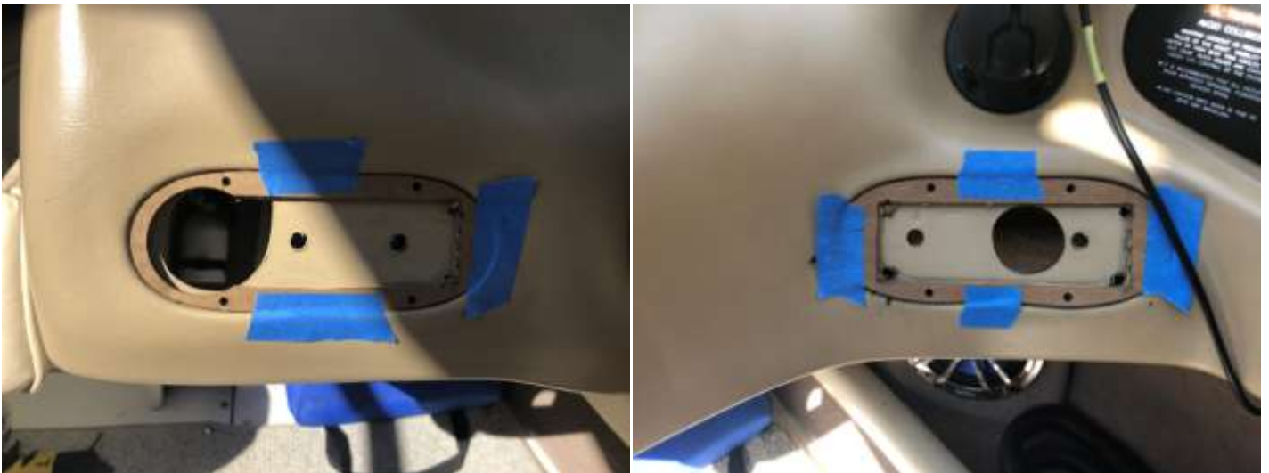
Figure 15: After drilling all the holes I removed the rectangular cut out center of the template. I did this to make cutting the opening easier.
