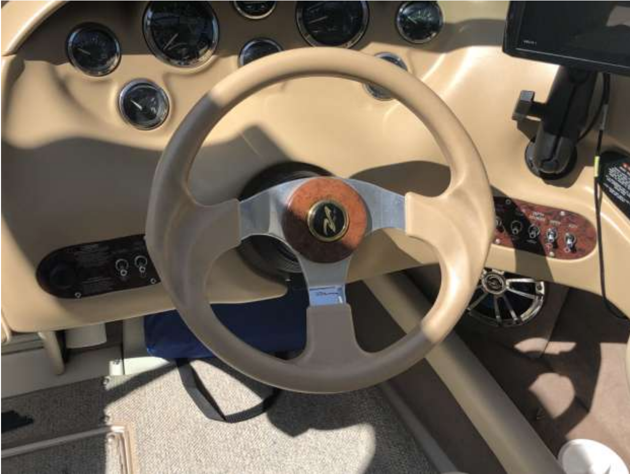
Figure 22: Finished! Note: There is a missing screw on the ignition panel. This is due to the original ignition switch cutout extending to far up. I will silicone in a screw so it looks complete.
